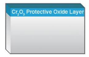
The chromium oxide layer is re-formed and protects against corrosion.
