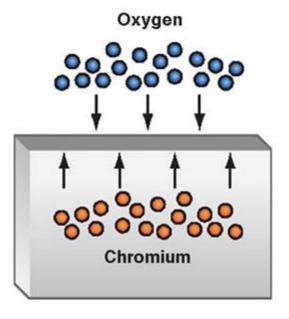
The chromium content in the stainless steel reacts with oxygen in ambient air.
